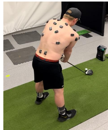
Figure 1: Surface EMG electrodes will be affixed to the participants bilaterally on their upper extremities and trunk.
