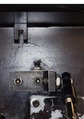
The L-shape bracket should not move to avoid any issues with drivability. The previous method of installation failed due to the repeated forces and vibrations that acted on it when the vehicle was in motion. The main problem was the misalignment of the wheel when the suspension was compressed. This would cause the zeroing of the wheel to be off affecting straight-line performance. To fix this issue we installed a new L-shape bracket that uses screws and nuts to secure the bracket.
