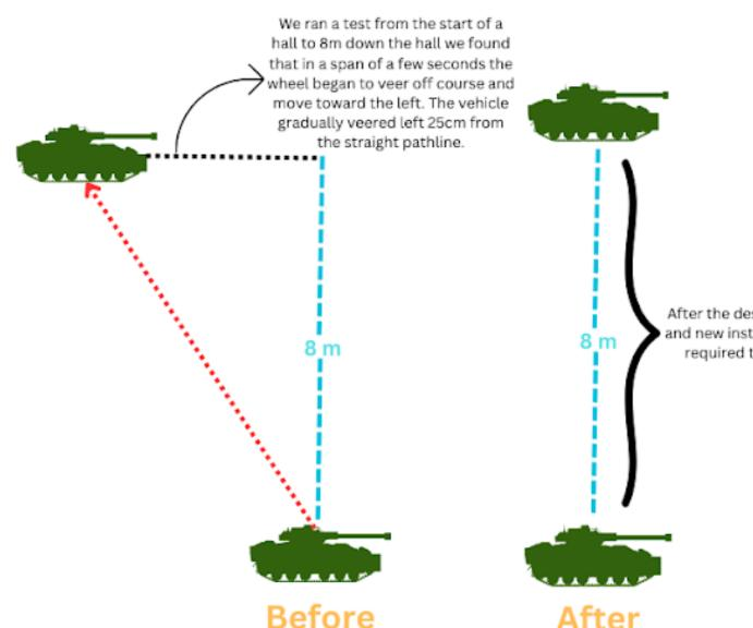
During a trial test before the enhancements and design changes to the vehicle it was discovered that the alignments of the wheels were off; as we ran a test from the start of a hall to 8 m down the hall we found that in a span of a few seconds, the wheel began to veer off course and move toward the left. The vehicle gradually veered left 25 cm from the straight path line, as shown in the figure above. These enhancements and design changes proved to be incredibly effective, as
