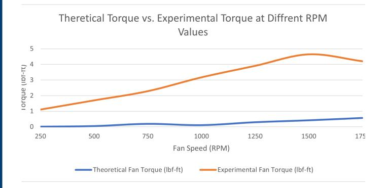
As expected, the results of the experimental torque far exceed the results of the theoretical torque, as the CFD simulations did not account for the friction losses in the prototype model. The prototype provides a scalable glimpse into the torque requirements of the 100% fan.
