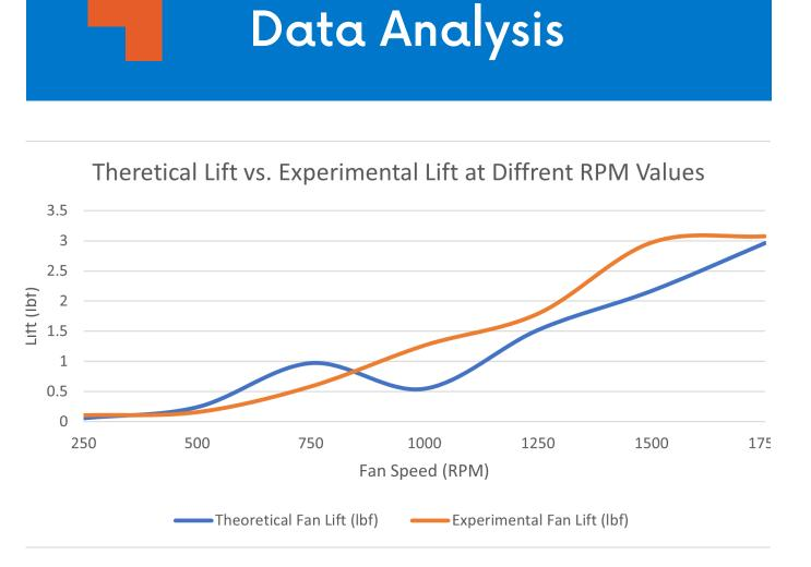
As seen in the chart above the experimental lift and the theoretical lift begin to converge around 3.1 lbf, at 1750 RPM. This indicates that the test data is relatively accurate and this model can be used to reliably predict the produced lift.
