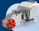
Motors //Rotates and also can measure the degree of rotation. Should be used for moving your robot around
