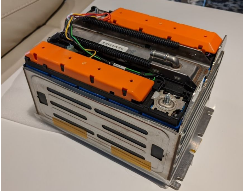
Fig 6: FIAT 500e Battery Module
