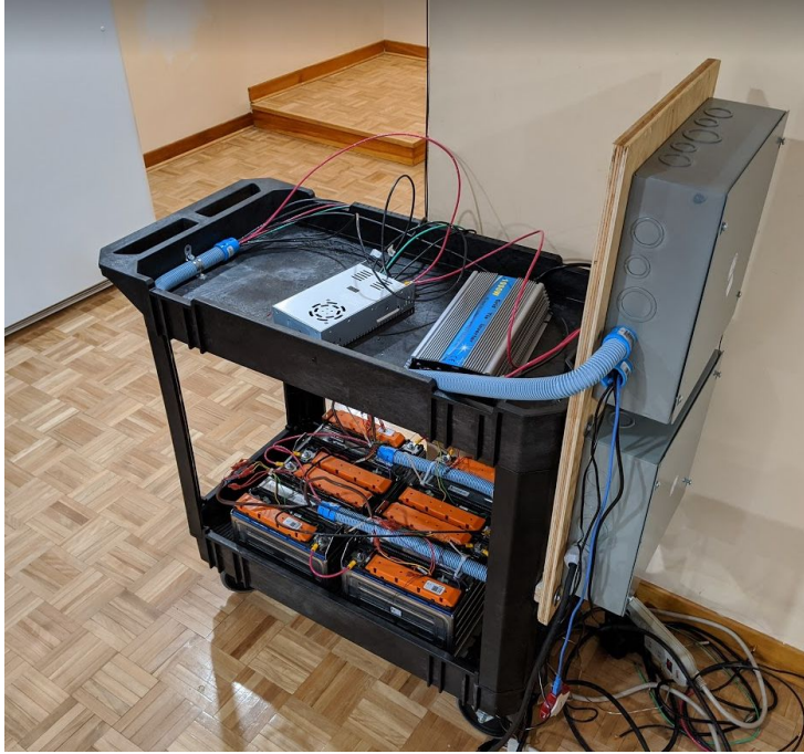
Fig 3: Our Peak Shaving System Reusing Used Fiat 500e Batteries
