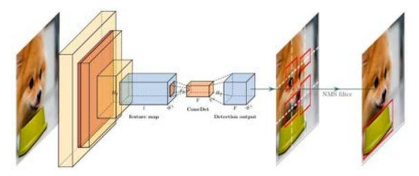
Figure 3: SqueezeDet pipeline. The feature map is of size  $W_fH_ff$ , where  $W_f$  and  $H_f$  refer to the width and height of the feature map, respectively, and f represents the number of channels. The output of the ConvDet, a  $F_w \times F_h$  convolution, is of size  $F := K \times (5 + C)$ . It is then trained to compute the class probability and the values associated with the bounding box at each grid center.
