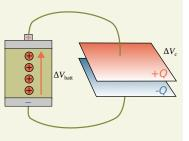
Capacitors in Series When connected in series, capacitors have the same charge Q but different voltages. Capacitors add in inverse:
