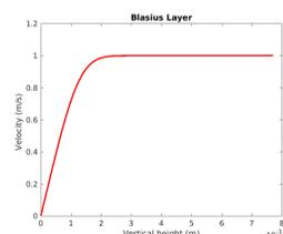
Fig. 1: The change in velocity due to the presence of a Blasius layer.
