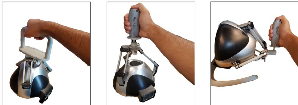
The devices can provide force feedback which allows the doctor and patient to feel a resistance if one or the other deviates from a motion path.
