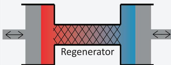
The addition of a *perfect* regenerator to a hot air engine allows the theoretical efficiency to approach that of the Carnot cycle, the highest possible efficiency for a heat engine.
