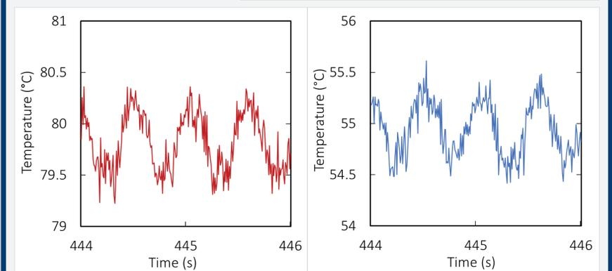
An equal temperature variation amplitude of 1°C was measured in each sub-regenerator at steady state.
