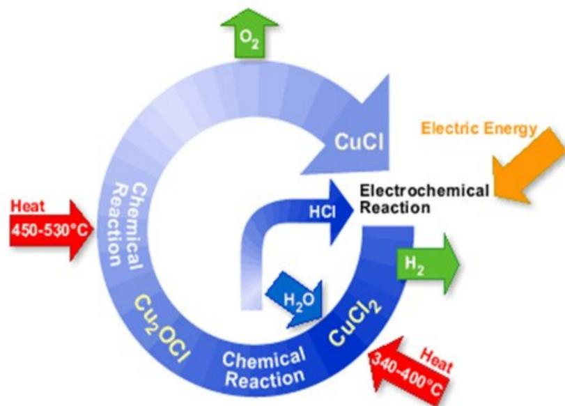
Figure 1: Engineering scaled schematic of copper-chlorine cycle
