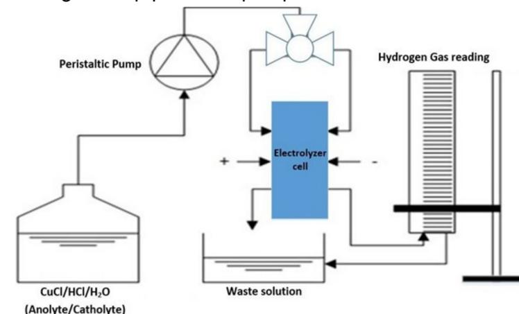
Figure 5: Schematic diagram of the electrochemical cell
