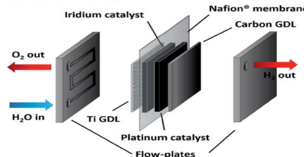
Figure 3: Electrolyzer setup with 3-layer membrane electrode assembly (MEA) and a Proton exchange membrane (PEM) -Nafion 115
