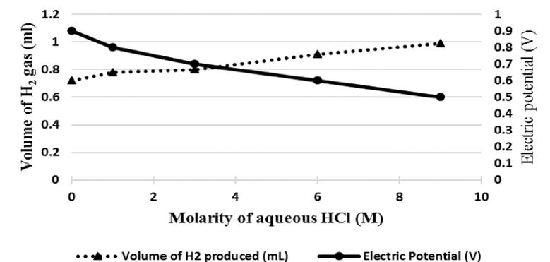
Figure 6: Relation between volume of  $\text{H}_2(g)$  with potential voltage drop and changing molarity of HCl
