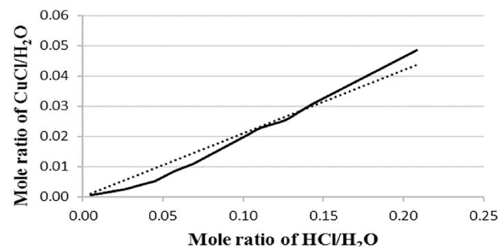
Figure 4: Solubility of CuCl powder in  $\text{HCl}_{(aq)}$  solution at 25 °C
