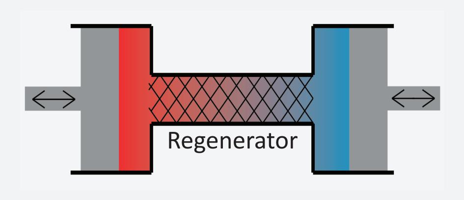
The addition of a *perfect* regenerator to a hot air engine allows the theoretical efficiency to approach that of the Carnot cycle, the highest possible efficiency for a heat engine.
