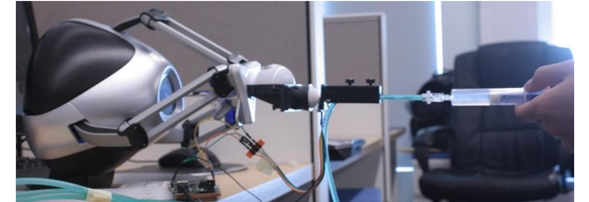
The Novint Falcon haptic device was augmented with a custom mount for a real epidural needle, and a gyroscope to allow orientation control.
