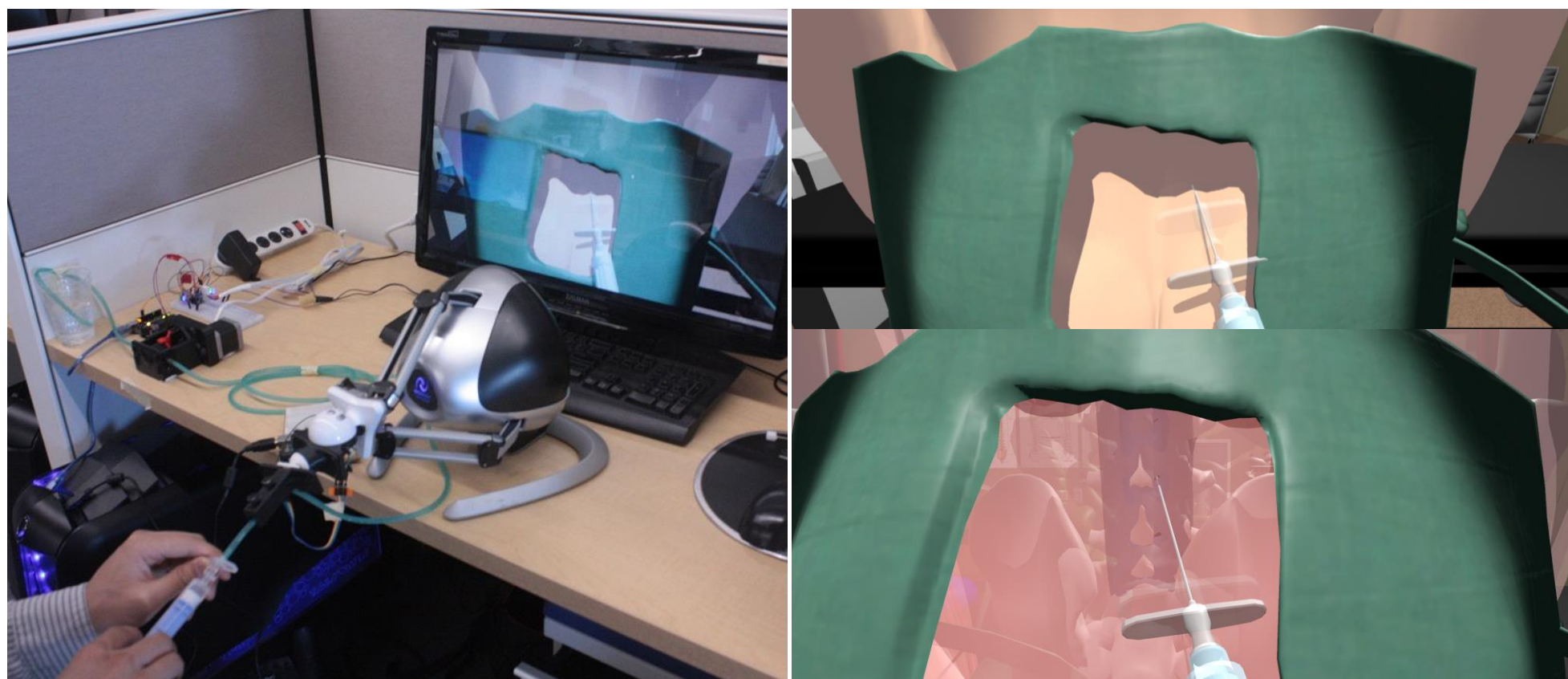
The user interacts with a haptic interface. Users can feel physical forces from the simulation
