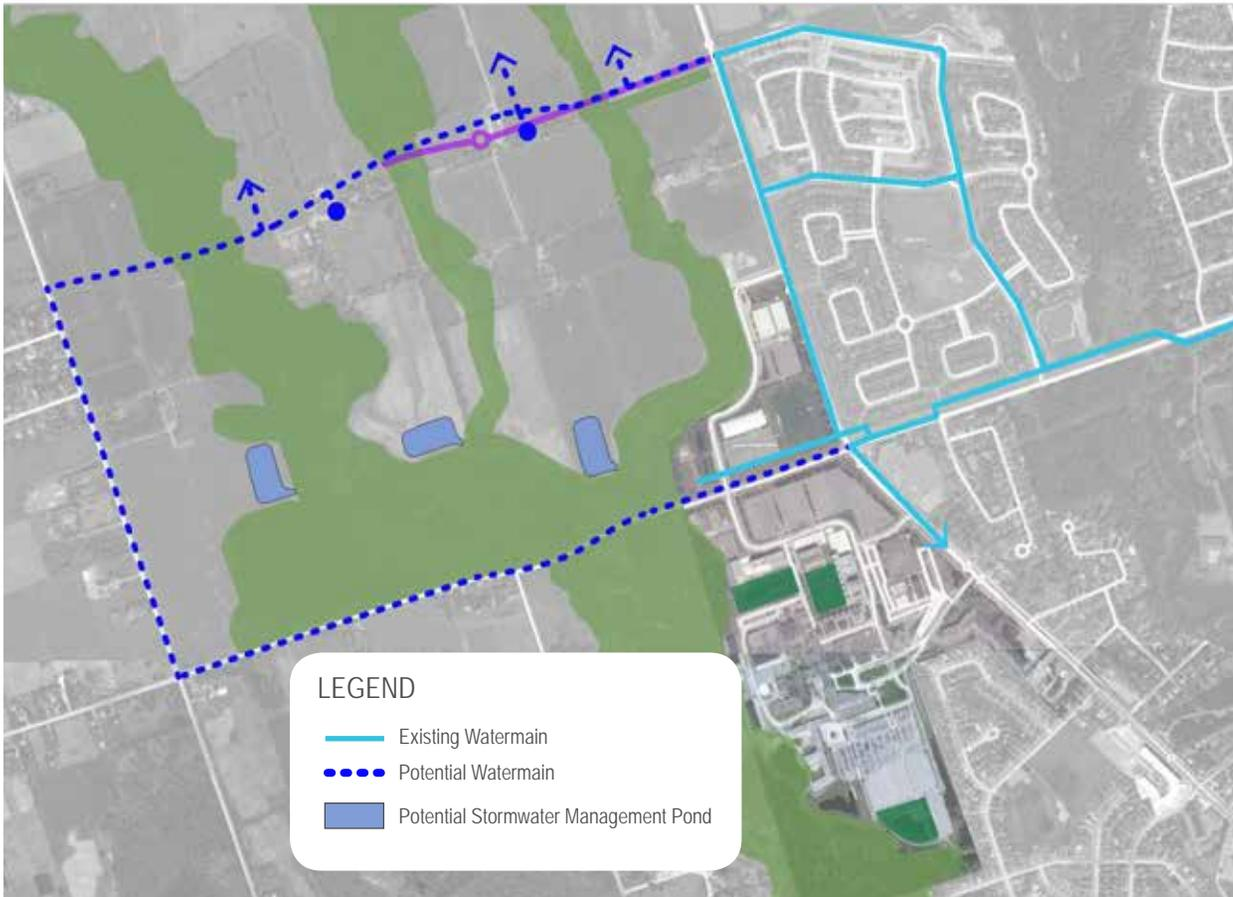
Figure 7.2 - Existing and Potential Water Servicing and Stormwater Management
