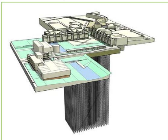
**Figure 1: Rendering of UOIT's Geothermal System**
