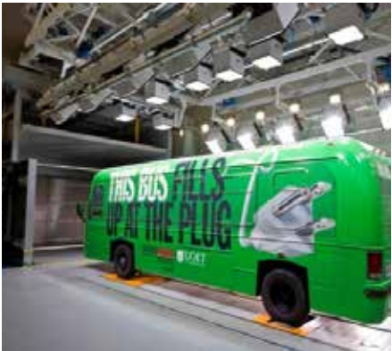
Solar array arranged for a bus (13 m 2 nozzle and 22 m 2 canopy)
