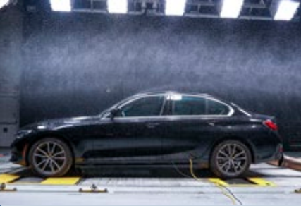
Blowing rain intrusion test
