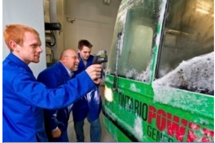
Measuring freezing rain on a bus
