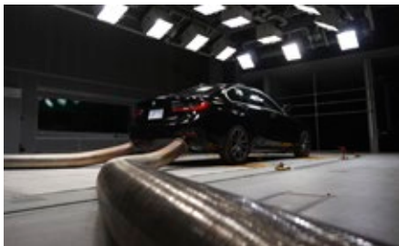
Dual closed-pipe vehicle exhaust extraction system
