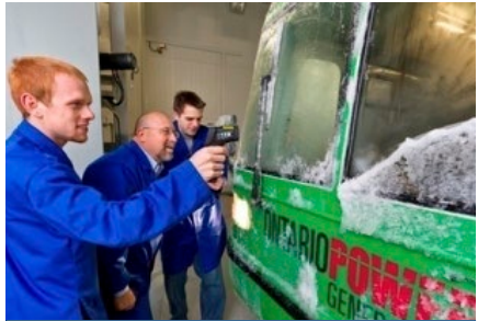
Measuring freezing rain on a bus
