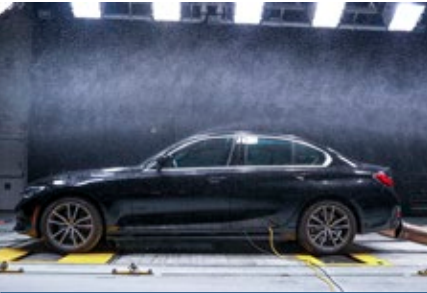
Blowing rain intrusion test
