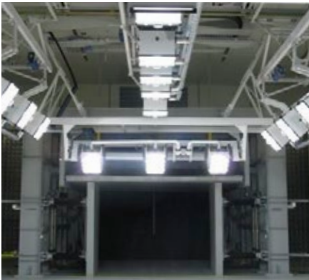
Solar array showing front illumination (9.3 m 2 nozzle)
