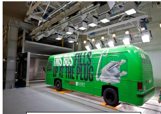
Solar array arranged for a bus (13m 2 nozzle and 22m 2 canopy)
