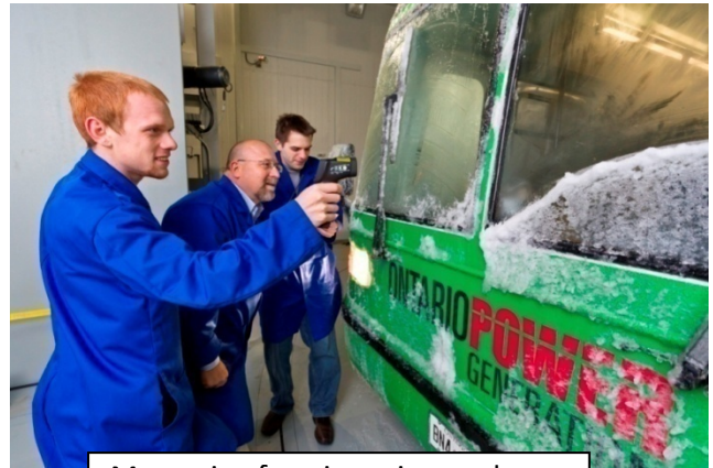
Measuring freezing rain on a bus
