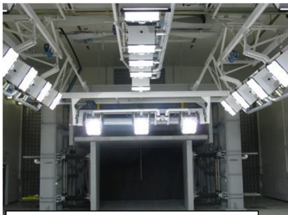
Solar array showing front illumination (9.3m 2 nozzle)
