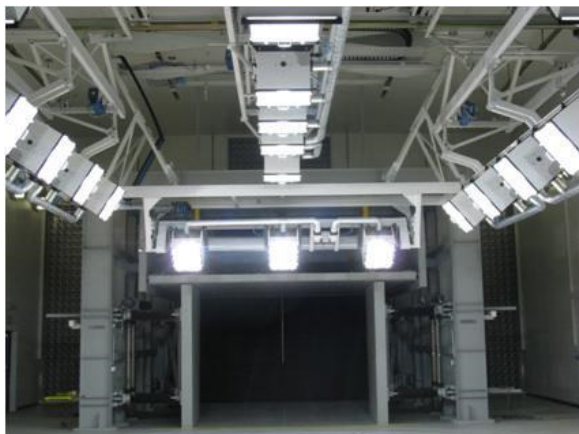
Solar array showing front illumination (9.3m 2 nozzle)
